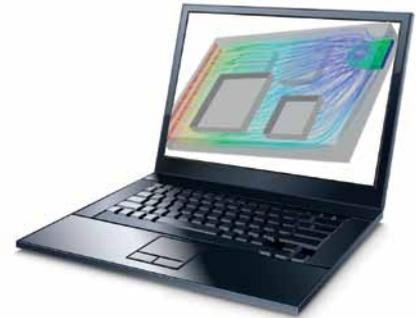
*When detecting unsatisfactory design performance, engineers modify the virtual design by changing the relevant design parameters and re-run the related simulation(s). Temperature peaks observed in a laptop can for instance be reduced by changing the location and characteristics of the laptop's active heat sink in the virtual prototyping model.*
