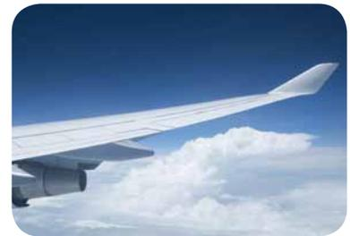
*Fuji Heavy Industries used Optimus to automate and couple FEM and CFD simulations to identify optimized aircraft winglet design configurations. Optimus realized a 1.2% reduction in aircraft takeoff weight for a typical mission profile at 1G cruise speed.*
