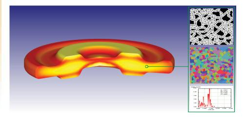
Microstructure modeling is used to predict residual stress and a wide range of mechanical properties. Scientific Forming Technologies Corporation is the leader in the development and application of microstructure modeling for research and industrial applications, as shown with the Cellular Automata (CA) model using the RVE method.
