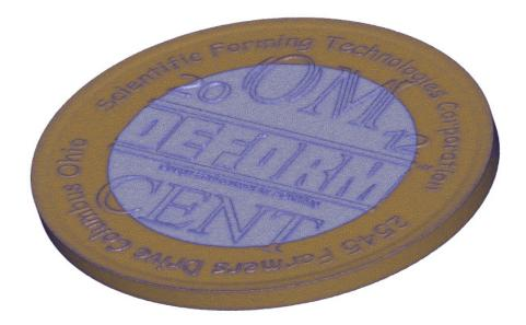
The core and rim of the bimetallic coin, shown above, were coined and mechanically joined together within a single operation. The multiple deforming body, advanced meshing and arbitrary capabilities of DEFORM-3D were required for such a complex simulation. Each body was modeled with over one million elements.
