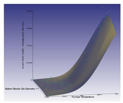
DEFORM Premier provides very powerful DOE and optimization capabilities to run multiple simulations with controlled process variation. DOE allows the user to define a test matrix using a full factorial or statistical sampling (Latin Hypercube) in advance. Optimization allows the system to fine a best process within defined constraints. A custom postprocessor automates much of the data mining and displays results in a usable format.
