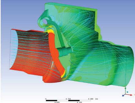
ANSYS CFX® software results show areas of turbulence inside the valve body, indicating areas that could be modified to reduce pressure losses. The contours represent velocity. ANSYS CFD and ANSYS DesignXplorer were used to optimize the design. *Courtesy Cameron.*
