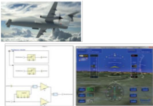
For this unmanned airborne vehicle, ANSYS SCADE automatically created a program source code with over 100,000 lines compliant with the aerospace safety standards.
