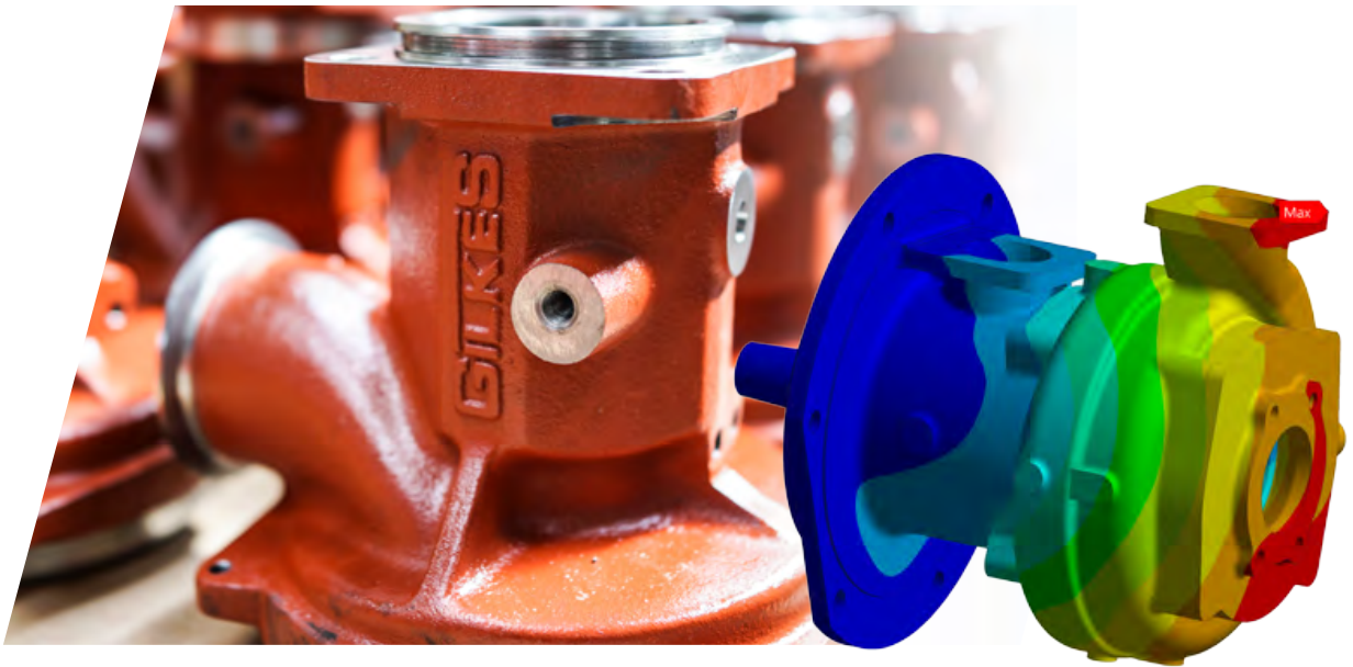
Gilkes cooling pumps on the shop floor (left) and ANSYS structural simulation of a dual-circuit marine pump (right)
